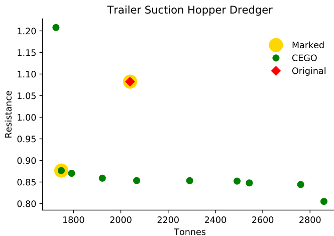
Figure 6.2: Obtained non-dominated design variations and original design. The marked solutions are the original solution and the most interesting optimized solution.
