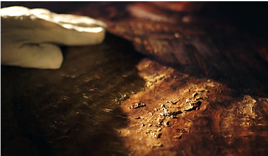
Figure I - 1. 3D printed detail (Isaak's sleeve) Rembrandt van Rijn's, The Jewish Bride , 1665, oil on canvas, 121 x 165.5 cm, Rijksmuseum, Amsterdam, inv. no. SK-C-216, material jetting / elevated printing, PLA on an aluminum base, Canon Production Printing BV (Venlo), 2015 © Clemens Weijkamp, 2015
