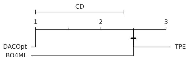
Figure 8.9: Comparison of all optimization algorithms compared to each other using Nemenyi test with a 5% significance level.
