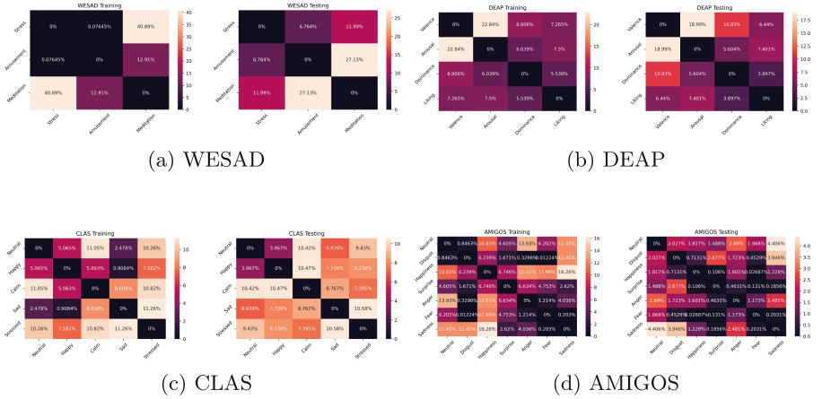
Fig. 4. Distance increase when using the novel cost function over MSE expressed as a percentage for training and testing data (LOSO) for the minimum distance between classes.
