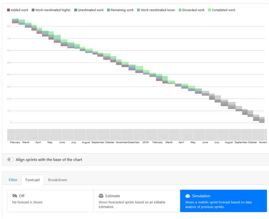
Figure 5.26: Product backlog burndown chart showing a Monte Carlo simulation of future sprints.
