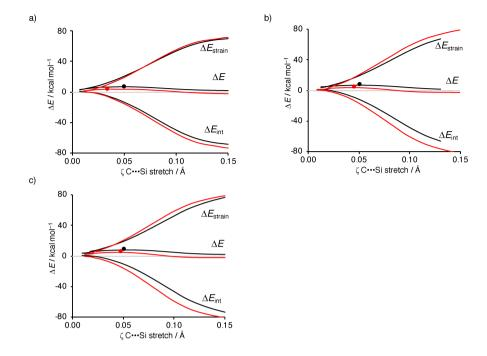
Figure S3. Activation strain model for the  $S_E2$ ' reactions of allyltrimethylsilane + cation 5 with gg rotamer (a), gt rotamer (b), tg rotamer (c) via the top face-attack (black: chair-like TS) and bottom face-attack (red: chair-like TS), where the energy values are plotted along the IRC projected on the C•••Si bond stretch. Computed at COSMO(CH<sub>2</sub>Cl<sub>2</sub>)-ZORA-B3LYP/TZ2P//PCM(CH<sub>2</sub>Cl<sub>2</sub>)-B3LYP/6-311G(d,p).
