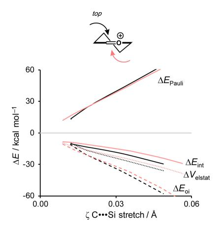
Figure S4. Energy decomposition analysis for the  $S_E2$ ' reactions of allyltrimethylsilane and cation 1 via the top face-attack (black: chair-like TS) and bottom face-attack (pink: twist boat-like TS), where the energy values are plotted to the transition state (indicated by a dot), along the IRC projected on the  $C \bullet \bullet \bullet \bullet$  Si bond stretch.
