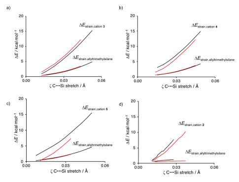
Figure S6. Strain decomposition for the  $S_EZ'$  reactions of allyltrimethylsilane + cation 3 (a), 4 (b), 5 (c), and 2 (d) via the top face-attack (black: chair-like TS) and bottom face-attack (red: chair-like TS), where the energy values are plotted along the IRC projected on the C•••Si bond stretch. Computed at COSMO(CH<sub>2</sub>Cl<sub>2</sub>)-ZORA-B3LYP/TZ2P//PCM(CH<sub>2</sub>Cl<sub>2</sub>)-B3LYP/6-311G(d,p).
