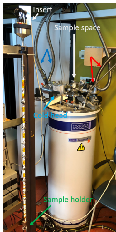
Figure 2.1: A photo of Teslatron in the lab. Key elements are marked in the photo. The blue arrows indicate the high-pressure helium circuit, whereas the red arrows point to the low-pressure circuit.
