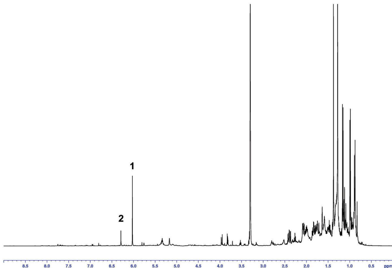
**Figure 2.** Typical  $^1\text{H}$ -NMR spectrum of an *A. annua* extract: 1 = the singlet from H-12 of ART at 6.015 ppm used for quantitation and 2 = the singlet from two symmetric protons at H-2 and H-3 of maleic acid at 6.280 ppm.
