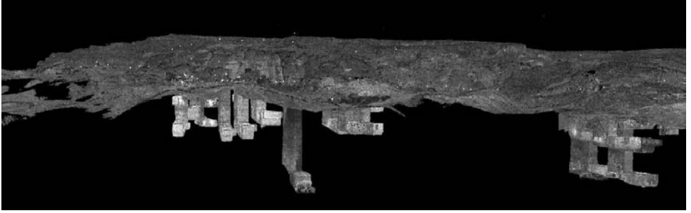
FIGURE 20.4 Screen shot of the point cloud of Zone 2, showing both the above ground landscape as well as the subterranean shafts and burial chambers
