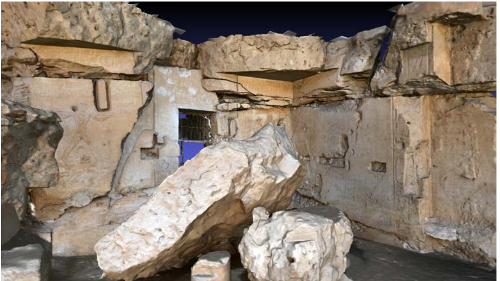
FIGURE 20.5 Screen shot of the mesh model of Djehutihotep's outer chamber obtained by combining TLS with photogrammetry
