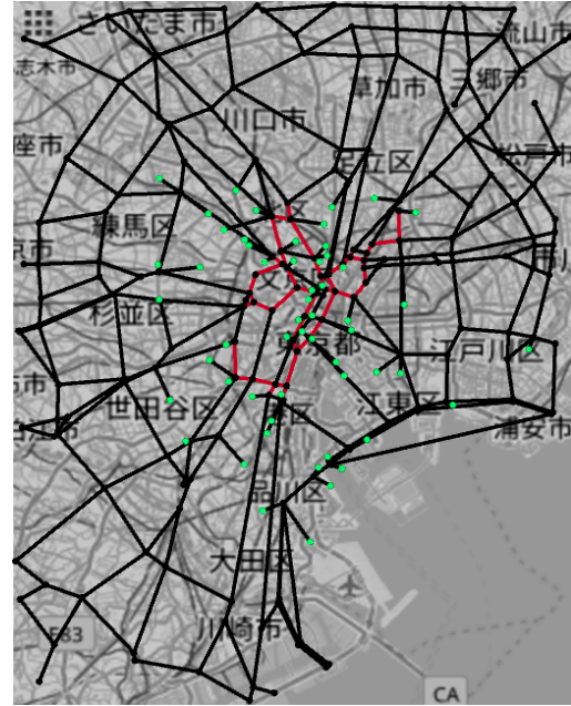
Fig. 6. Visualisation of the road network, as an overlay on a map of Tokyo, with edges coloured according to their associated variable costs. Red edges have high costs, while black edges have a cost of 0. Map source: OpenStreetMap [20].
