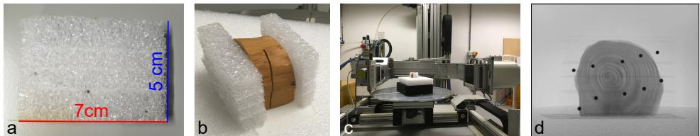
**Figure A.3: Preparing the markerholder.** a) Including markers in foam. b) Placing foam next to the wooden block. c) Placing the wooden block and markerholder on the rotation stage at the Rijksmuseum. d) Resulting radiograph in the Rijksmuseum facility.
