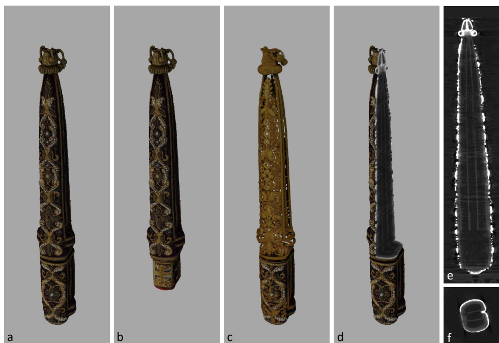
Figure 5.8: a) Surface scan of the cutlery case and lid - aligned using the CT of the full object, b) surface scan of the case only, c) CT volume representation and surface scan of lid, d) surface scan, cut open to show the CT slices, e) corresponding vertical slice, f) corresponding horizontal slice.
