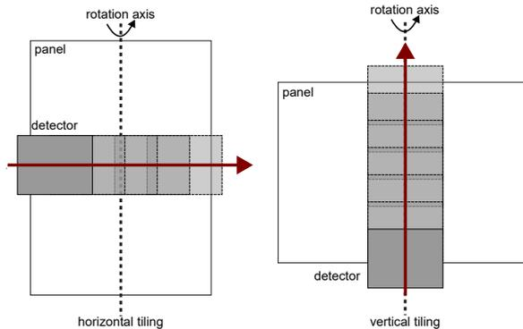
**Figure 1.7:** Schematic indicating the two tiling modes that were investigated for the scan of a panel painting, the panel is outlined in white and the detector in grey, with lighter grey indicating subsequent detector positions. Image adapted from [60].
