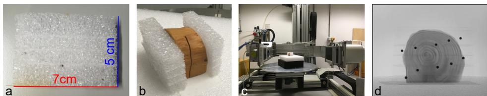
**Figure A.3: Preparing the markerholder.** a) Including markers in foam. b) Placing foam next to the wooden block. c) Placing the wooden block and markerholder on the rotation stage at the Rijksmuseum. d) Resulting radiograph in the Rijksmuseum facility.
