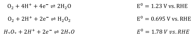
Scheme 1. Standard Electrode Potentials of the Different Catalytic Reactions Involved in the ORR, and Postulated Mechanism for the ORR and Hydrogen Peroxide Reduction Reaction (HPRR) Mediated by Cu-tmpa
