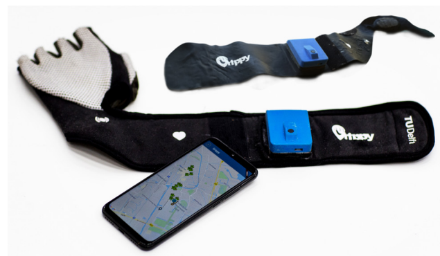
Figure 2. The Grippy prototype includes a physical glove (with a glove-shaped version and a strap-shaped version provided) connected to an app on a smartphone.
