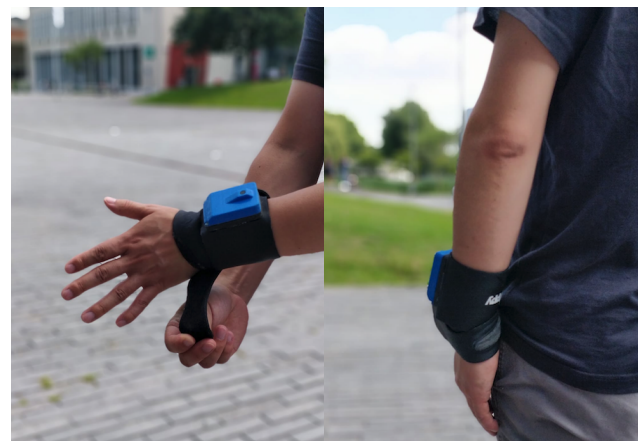
Figure 4. Illustration of how the flexible strap-shaped version of Grippy can be worn with the haptic wrapped up and fixed around the wrist.
