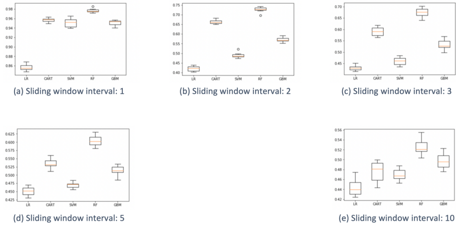
Figure 2.5: Accuracy of different classifiers in various sliding window intervals in order to predict whether a sequence contains a one- or a two- handed sign or not signing at all. At a sliding window interval of 1 (a), Random Forest shows the highest accuracy.
