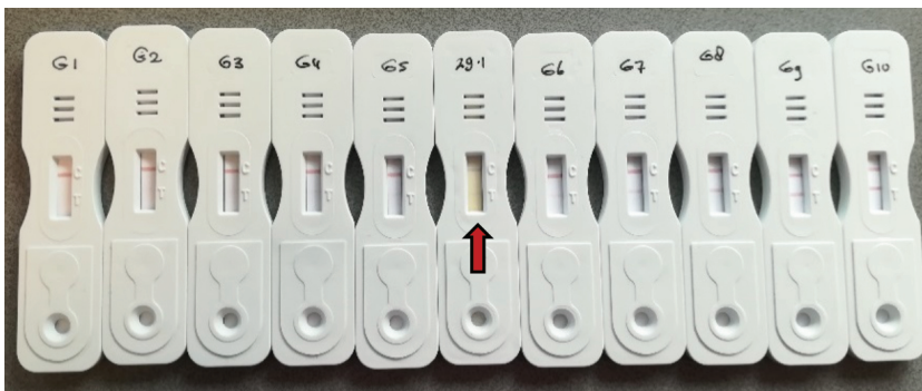
Figure 2. Example of scoring a urine sample using the G-scores. The arrow indicates the cassette to be scored, which is placed in between the G-scores that resemble the intensity of the test line in order to select the best matching G-score.
