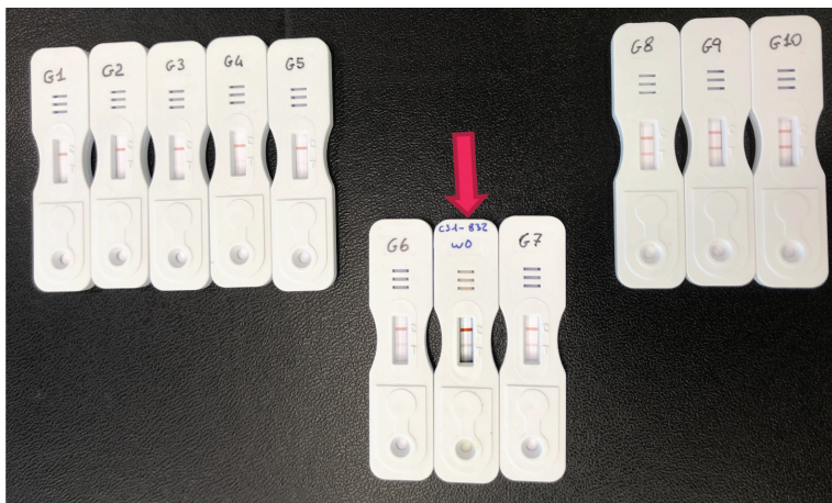
Figure 9. Scoring a cassette by looking at the test line and comparing with the set of G-scores.
