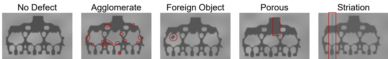
Figure 7: Anomaly types included in the synthetic data (red: highlighted location of anomaly). Agglomerate: accumulation of unwanted loose components into a solid compound. Foreign object: unknown objects on the printed. Porous: temperature difference in the direction of print head movement. Striation: vertical striations from excess binder, sand or nozzle-clogging.
