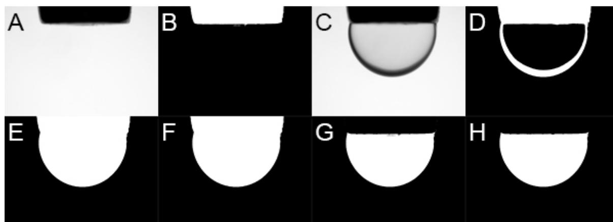
**Figure S1.** Image processing steps for the droplet volume calculation algorithm, in order: A) background image of the needle; B) binarized needle image; C) original droplet image; D) binarization with threshold; E) hole-filling; F) particle filter to remove unconnected pixels; G) needle subtraction; H) particle filter to remove unconnected pixels.
