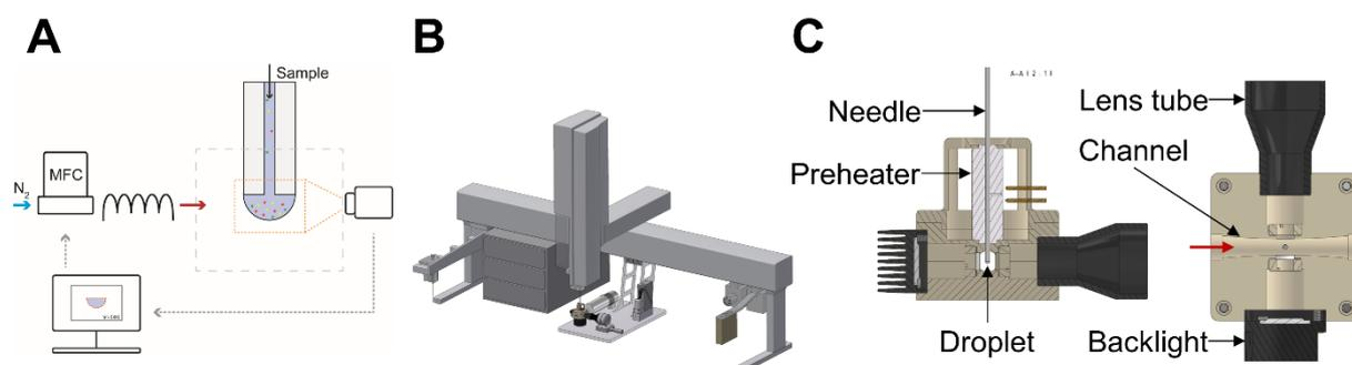
**Figure 1.** Schematic overview of the automated droplet evaporation preconcentration module. A) Schematic representation of the evaporative preconcentration principle; B) CTC PAL3 robotic autosampler with integrated droplet evaporation module; C) Detailed cross-sections of the evaporation chamber showing the channel cross-section at the droplet (left) and the lofted profile of the gas flow channel (right).
