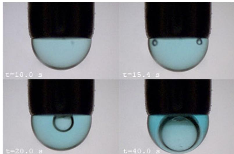
**Figure S4.** Formation of a vapor bubbles inside the evaporating droplet. Stills from the preconcentration of 8.0 to 0.8  $\mu\text{L}$  of 5.0  $\mu\text{g}/\text{mL}$  methylene blue in 30:70 water:acetonitrile, with a gas inflow temperature of 150-165  $^{\circ}\text{C}$  and an evaporation rate of 6  $\mu\text{L}/\text{min}$ .
