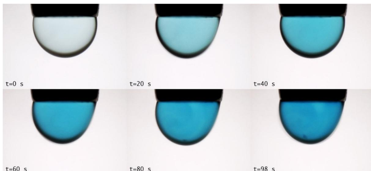
**Figure 3.** Fifteen-fold pre-concentration (from 12 to 0.8  $\mu\text{L}$ ) of methylene blue in water:MeOH 1:1 (v:v) solution with an initial concentration of 5  $\mu\text{g}/\text{mL}$  in ca. 3 min.
