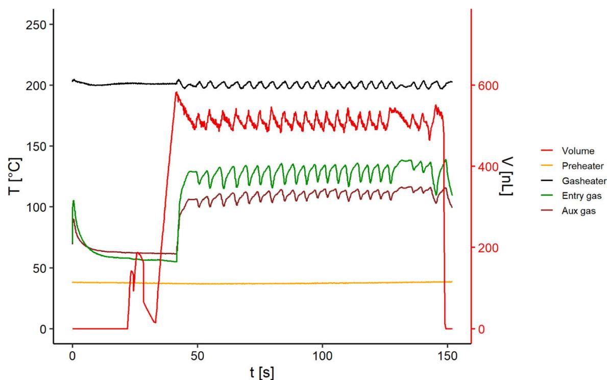
**Figure S2.** Droplet volume and (gas) temperatures recorded during the solvent evaporation from a 500 nL droplet of methylene blue in 50% MeOH at a rate of 6  $\mu\text{L}/\text{min}$ .. The gas temperatures as well as the droplet volume show a mild oscillation as response to the fluctuating gas flow rate, regulated by the PI feedback control loop. The droplet volume remains stable within 50 nL of the setpoint value throughout the process.
