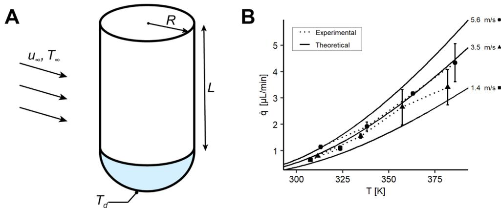
**Figure 2.** A) Schematic of the hemispherical droplet on a cylindrical rod; B) Theoretical and experimental evaporation rates of a hemispherical water droplet with a base radius of 1.3 mm at free stream velocities of 1.4-5.6 m/s and temperatures of 300-393 K.
