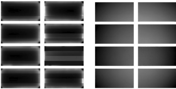
Figure 8. Left-hand panel: The raw flat-field exposure with severe scatter-light signal. Right-hand panel: The scatter-light corrected flat-fields preserving both the low frequency component of the vignetting and the high frequency of the pixel-to-pixel variations.
