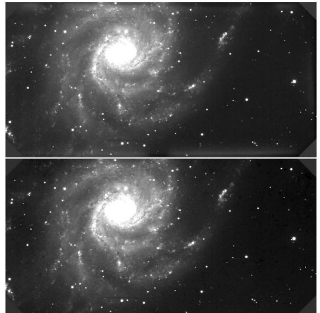
Figure 6. Top panel: A rare science frame with a very extended source (M101) without scatter-light correction. Bottom panel: A sky-flat corrected science image preserving the light from extended sources.
