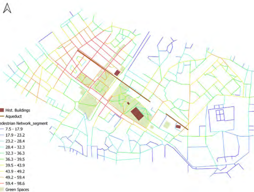
Figure 2: Angular Segment Integration Analysis r300m - Existing Pedestrian Network
