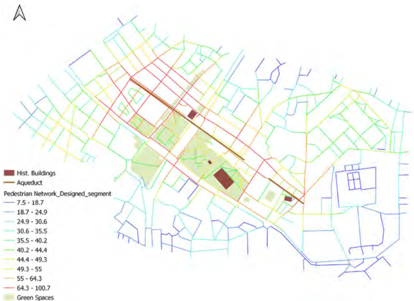
Figure 4. Angular Segment Integration Analysis r300m - Proposed Network
