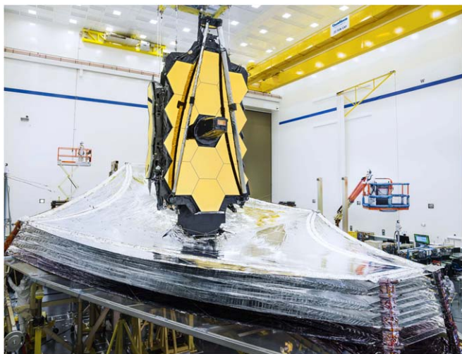
Figure 1. JWST in the Northrop Grumman cleanroom following a sunshield deployment test.
