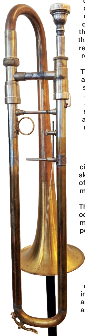
Image 1: Slide trumpet constructed by the author.
