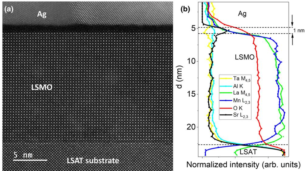
FIG. 5. (a) High-angle annular dark field image, made by scanning transmission electron microscopy, of an LSAT/LSMO/Ag sample. It shows the epitaxial LSAT/LSMO interface and the disordered LSMO/Ag interface. Two different grains are visible in the Ag layer. (b) Averaged electron energy loss chemical map showing the Ta  $M_{4,5}$ , Al K, La  $M_{4,5}$ , Mn  $L_{2,3}$ , O K, and Sr  $L_{2,3}$  intensity profiles of the layers. Dashed lines indicate the LSAT/LSMO and LSMO/Ag interfaces.
