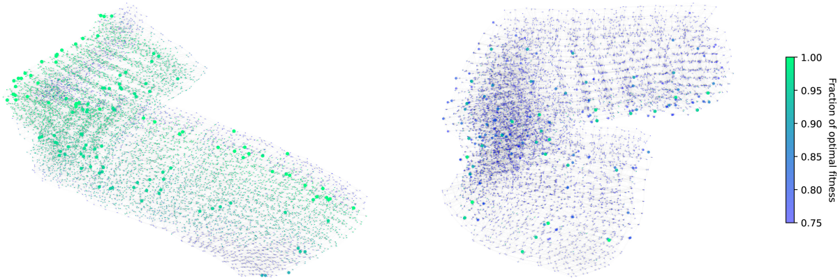
Fig. 6. FFGs of PnPoly kernel search spaces of the (left) NVidia Titan RTX, and (right) NVidia GTX 1080Ti. Each node is a point in the search space. There is a directed edge between neighboring points from higher to lower fitness. Points are colored within a fitness range of +25% with respect to the global minimal fitness (global minimum in green), i.e., each point is colored by its fraction of optimal fitness, and points with a fraction below 0.75 are given the same color. Local minima are represented as larger nodes.
