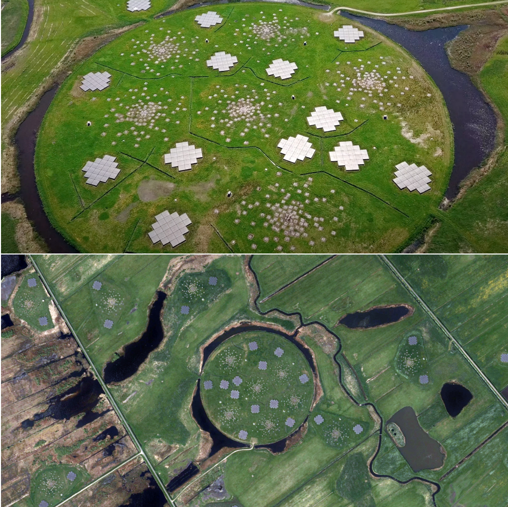
Figure 1.6: The LOFAR’s core lies in the moors of Drenthe, one of the Netherlands’ northern provinces. The Superterp , shown here, is a circular, elevated island with a diameter of 320 metres that contains 6 of the 24 core stations. Each core station comprises 96 low-band antennae and two sets of 24 high-band antenna tiles. The data underlying this thesis were collected using the high-band antennae only. In the bottom image, north is at the top. From: ASTRON drone footage, 2018 (top); Kadaster aerial imagery, 2022 (bottom)
