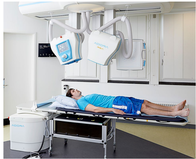
Fig. 2 The DR-system set-up for shoulder RSA with the patient in supine position and arms resting with the palm of the hand against the bed. The calibration box is positioned lengthwise to the examination table
