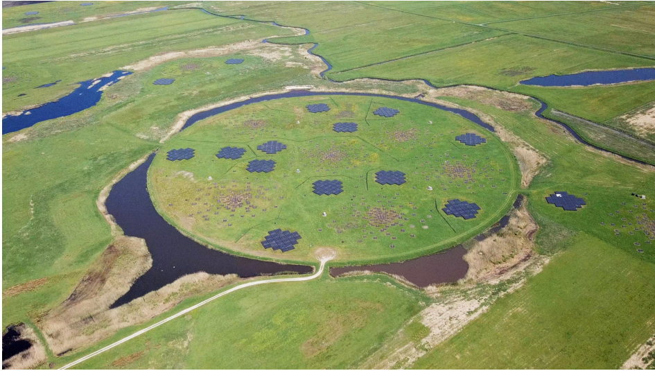
Figure 1.6: The core of the LOw Frequency ARray (LOFAR), known as the “superterp”. The LBA stations are the more “randomly” distributed wire dipoles, whereas the HBA stations are the gridded sets of dark grey boxes. Image credit: LOFAR.
