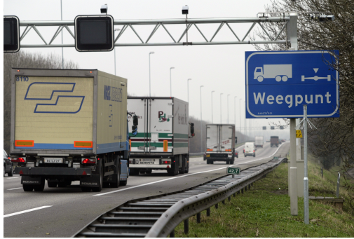
Figure 1.4: The Weigh-In-Motion system.
