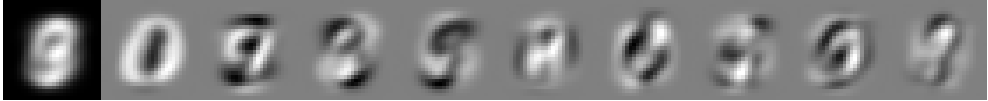
Figure 3.3: The mean values (left) and first 9 principal components of the MNIST dataset. (Greyscale ranges have been rescaled for maximum visibility.)
