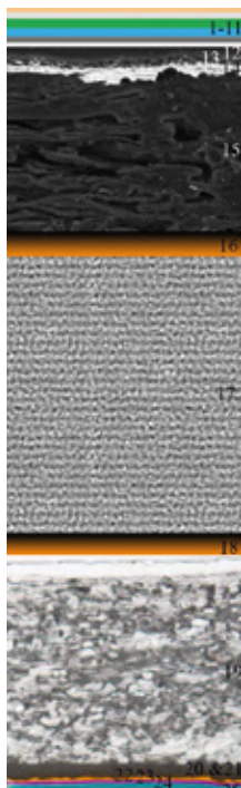
FIGURE 3.9. Imagined cross section of Dutch Grey : varnish (1), layers of the alkyd paints (2–11), four layers of the silver gelatin print (12–15), double-sided adhesive (16), foam core (17), double-sided adhesive (18), paper base including the backing of the chromogenic photograph (19), solid-liquid interface (20 & 21), yellow layer (22), magenta layer (23), cyan layer (24), protective layer (25). Not included are the three thin interlayers with UV absorbers and scavenger between the layers 22 and 23, 23 and 24, and 24 and 25.
