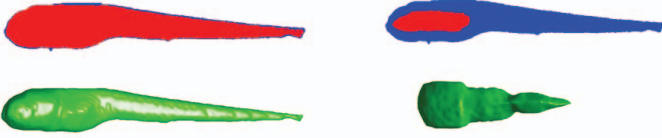
Fig. 3. Camera configuration effects for silhouette-based 3D model reconstruction. Blue area: ground-truth silhouette. Red area: overlap between the projected and the ground-truth mask. Green surface: reconstructed shape. Left column: optimal camera configuration gives maximal overlap area and obtains natural shape. Right column: inaccurate camera configuration gives small overlap area and obtains poor shape.
