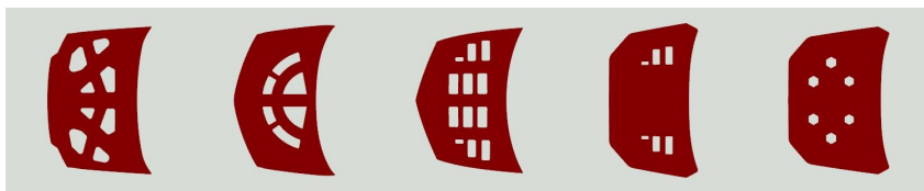
Figure 6.1: Example of variability in car hood designs in the data set. The variability is due to the introduction of features, e.g., pockets, cut outs, and ribs.
