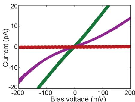
**Figure A3.10:** Current-voltage ( $IV$ ) characteristics measured after deposition of buffer without ferritin, at 4.2 K. Three different  $IV$  types are observed: device that remains open (red dots), tunneling-like (purple dots), linear behavior (green dots).
