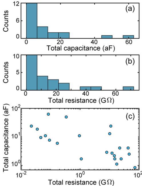
**Figure 3.6:** Total capacitances ( $C = C_1 + C_2$ ) and total resistances ( $R = R_1 + R_2$ ) calculated with the orthodox Coulomb blockade model for the 22 devices showing Coulomb-blockade at temperatures below 100 K. Table A3.10 contains the entire set of Coulomb blockade parameters used to model each device, at the lowest recorded temperature. (a) Total capacitance histogram. (b) Total resistance histogram. (c) Total capacitance plotted against the total resistance.
