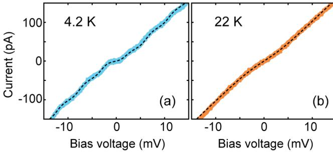
**Figure 3.5:** Experimental current-voltage characteristics acquired on device A1, at 4.2 K (light blue dots) and 22 K (orange dots). The black dashed lines indicate the calculated curves using the orthodox Coulomb blockade model with parameters:  $C_1 = 28$  aF,  $C_2 = 34.7$  aF,  $R_1 = 0.4$  M $\Omega$ ,  $R_2 = 0.08$  G $\Omega$ ,  $Q_0 = 0.15e$ .
