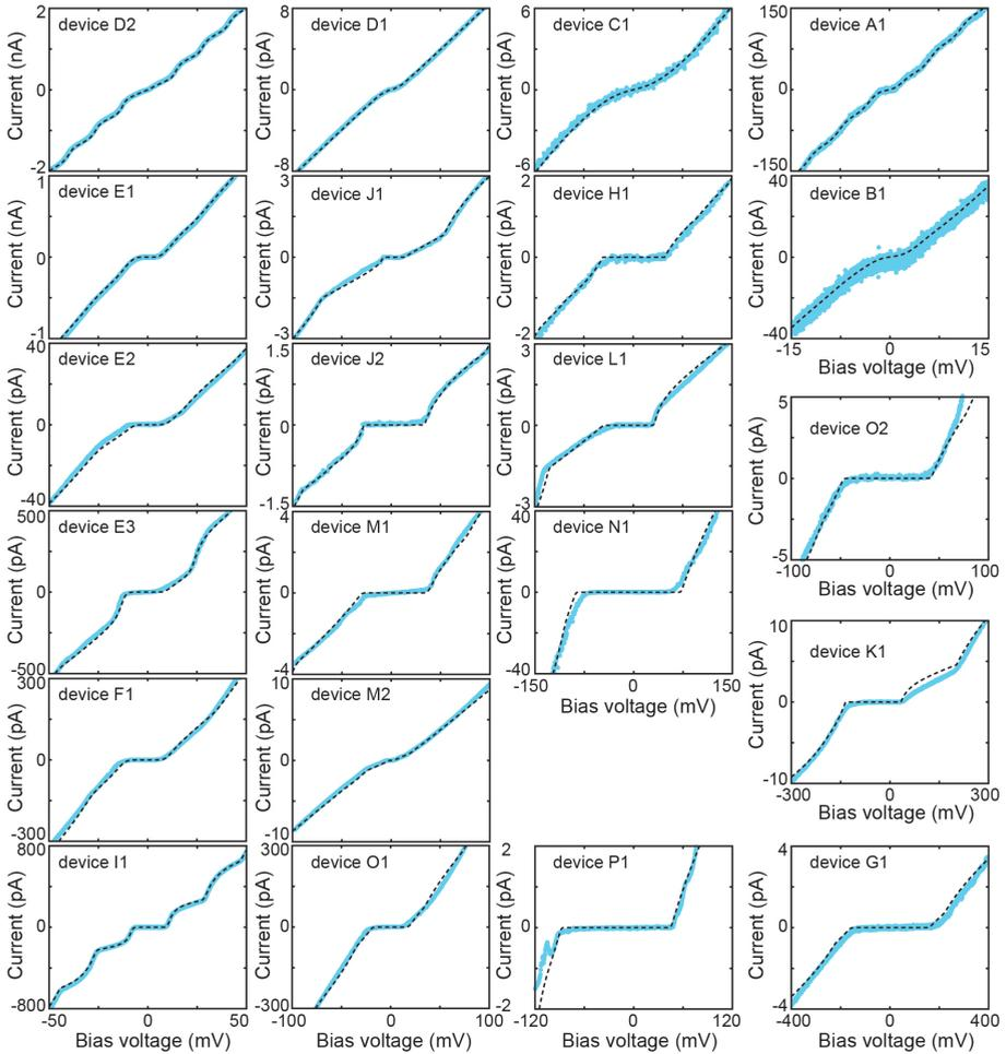
**Figure A3.11:** Low-temperature experimental current-voltage characteristics (blue dots) and the corresponding calculated curves using the orthodox Coulomb blockade model (black dashed lines) acquired on the 22 devices displaying Coulomb blockade-like features. The fit parameters and the temperature at which the measurement was performed are collected in Table A3.10.
