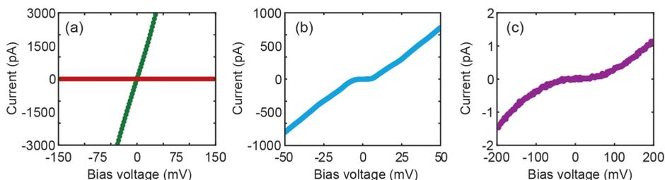
**Figure A3.9:** Examples of the four types of experimental current-voltage ( $IV$ ) characteristics measured after deposition of ferritin at 4.2 K;  $IV$ s are recorded by sweeping the voltage from negative to positive values, and vice versa. Note, the absence of hysteresis. (a) Device that remains open (red dots) and a device that shows a highly conductive linear behavior (green dots). (b) Device that shows Coulomb-blockade-like features. (c) Device that shows tunnelling-like behavior.
