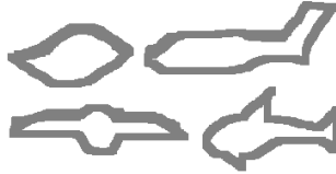
Fig. 2. Some examples of prototype templates of different objects. Gray area represents the space where connected component boundaries might be located.
