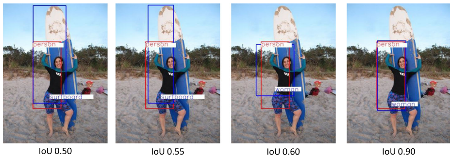
Fig. 4 IoU example: The red color box and blue color box come from MS COCO and Visual Genome, respectively, and the IoU value of two different boxes of the same object should be high
