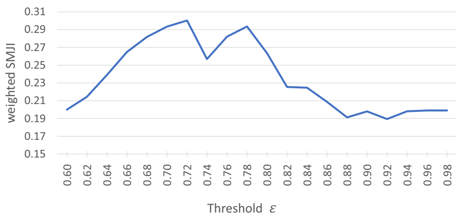
Fig. 5 The effect of \varepsilon in (2) on the performance of semantic mapping in terms of weighted SMJI on the FG-sCOCO validation set
