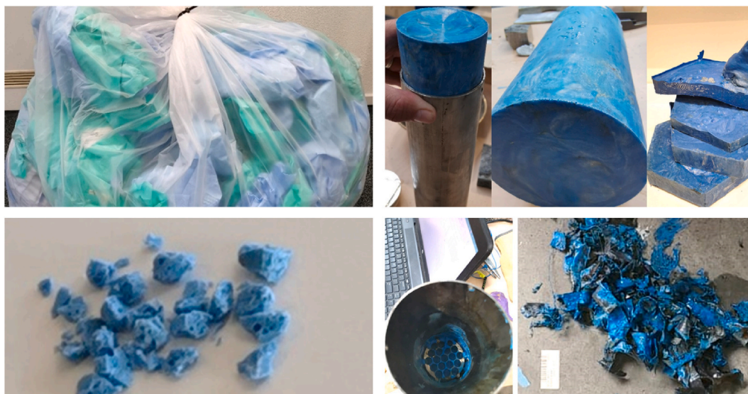
Fig. 2. Overview of different stages of material. From top left to bottom right: collected WP, melted WP formed into bars, granulated WP after melting, filter inside melting tube, and residue removed from filter used to make polluted dog-bones.
