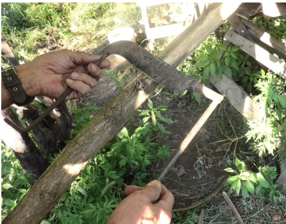
[Image 9: Dino's self-made scraping tool. 12/09/2019. Screenshot of videos taken by the author.]
