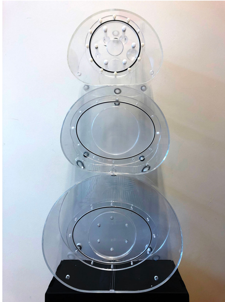
Fig. 1 The phantoms used to determine the RC. Upper phantom: NEMA IEC body phantom. Lower two phantoms: custom-made phantoms reflecting a larger body mass index (BMI, \text{kg}/\text{m}^2 ) of patients. Note that the lower two phantoms are depicted without spheres inset
