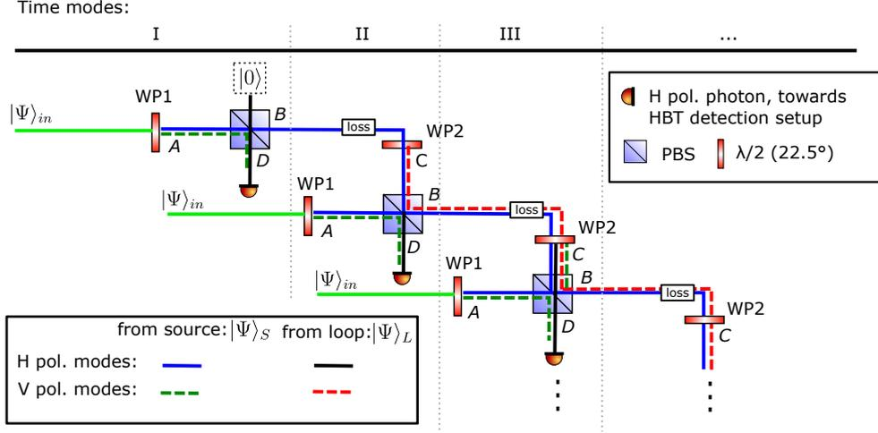
Figure 6.6: Flow chart of the computer algorithm to calculate  $g_{HH}^{(2)}(0)$ . It is an unfolded version of the real experiment where photons in mode  $D$  are sent to the HBT detection setup, each of these ports corresponds to a different time mode.
