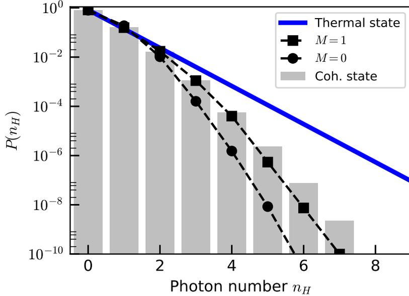
Figure 6.4: Comparison of the photon number distribution of a weak coherent state (bars) and thermal state (through blue line) with same mean photon number  $\bar{n} \approx 0.2$ , to the results from our theoretical model (squares for the case of indistinguishable photons,  $M = 1$ , and circles for the case of distinguishable photons,  $M = 0$ ). A fixed round-trip loss of 0.1 is included in both cases. The artificial state matches best to the weak coherent light state.
