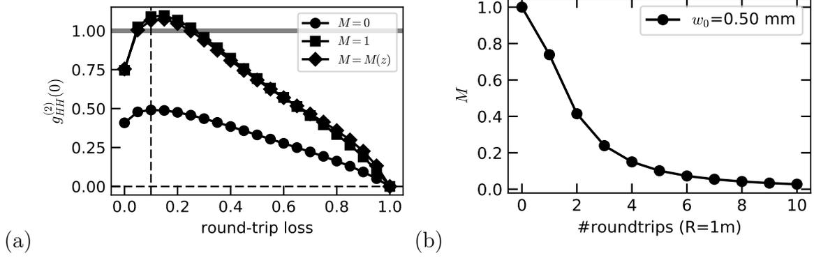
Figure 6.8: Effects of round-trip loss and diffraction. (a) Dependence of  $g_{HH}^{(2)}(0)$  on round-trip loss, for the case of fully distinguishable ( $M = 0$ ), indistinguishable ( $M = 1$ ) photons, as well as round-trip dependent indistinguishability due to diffraction. The vertical dashed line points to our experimental round trip loss of  $\sim 0.1$ . (b) Effect of gaussian mode diffraction on the distinguishability or wave function overlap  $M$ .
