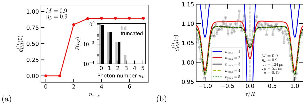
Figure 6.10: Influence of higher photon number states based on truncated computer simulations. (a) Dependence of  $g_{HH}^{(2)}(0)$  on the maximum photon number, the inset shows the full (gray) and truncated (black) simulated photon number distribution ( $M = 0.9$ ,  $\eta_L = 0.9$ ). (b) Comparison of differently truncated simulations to the experimental  $g_{HH}^{(2)}(\tau)$  data. At least 3 photons are needed to explain the experimental data.
