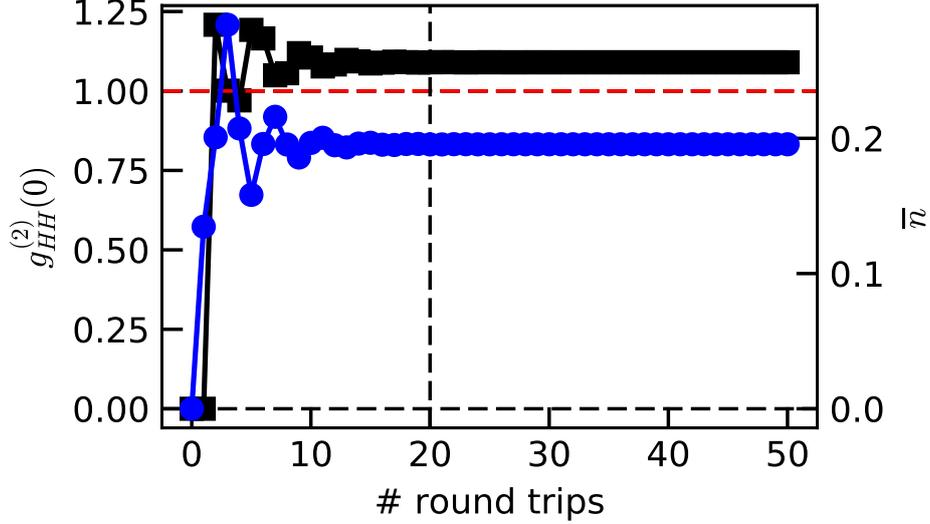
Figure 6.7: Correlation  $g_{HH}^{(2)}(0)$  (black) and average photon number  $\bar{n}$  (blue) as a function of the number of round trips for perfectly indistinguishable photons ( $M = 1$ ) and experimental round-trip loss  $\eta_L = 0.9$ . The vertical line shows our choice of 20 round trips where the field is sufficiently converged.
