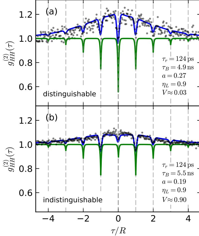
Figure 6.3: Photon correlations  $g_{HH}^{(2)}(\tau)$  (symbols) for misaligned loop (a,  $V \approx 0.03$ , distinguishable photons) and aligned loop (b,  $V \approx 0.9$ , indistinguishable photons) compared to the model predictions (blue curves). Raw coincidence counts corresponding to  $g_{HH}^{(2)}(\tau) = 1$  were 880 (a) and 9700 (b). The green curves show the model results for the case without spectral diffusion.
