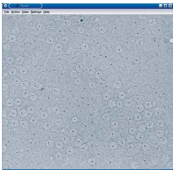
Fig. 4. Part of a micrograph of MS2 particles. The crosses show the initial coordinates determined in step 1 of the particle picking using the local variance method.
