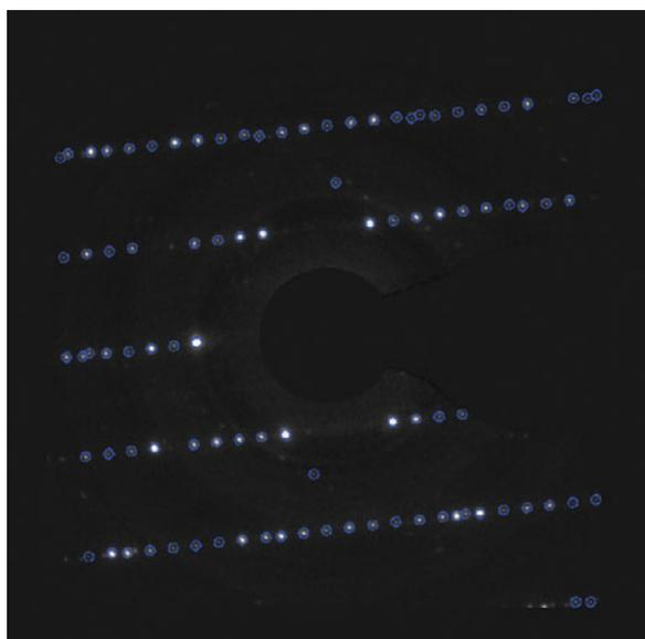
**Figure 3.** The result of image background removal, centering, and spot localization of the image in Figure 2a. Recognized diffraction spots are marked by circles.
