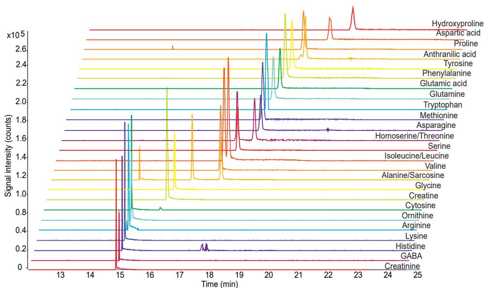
**Figure 2.** Extracted-ion electropherograms obtained by CE-MS from the analysis of 28 metabolites (5  $\mu\text{M}$ ) spiked in perfusate. Separation conditions: BGE, 10% acetic acid; sample injection volume 291 nL; ammonium hydroxide (concentration: 5%) pre-injection volume, 12 nL.
