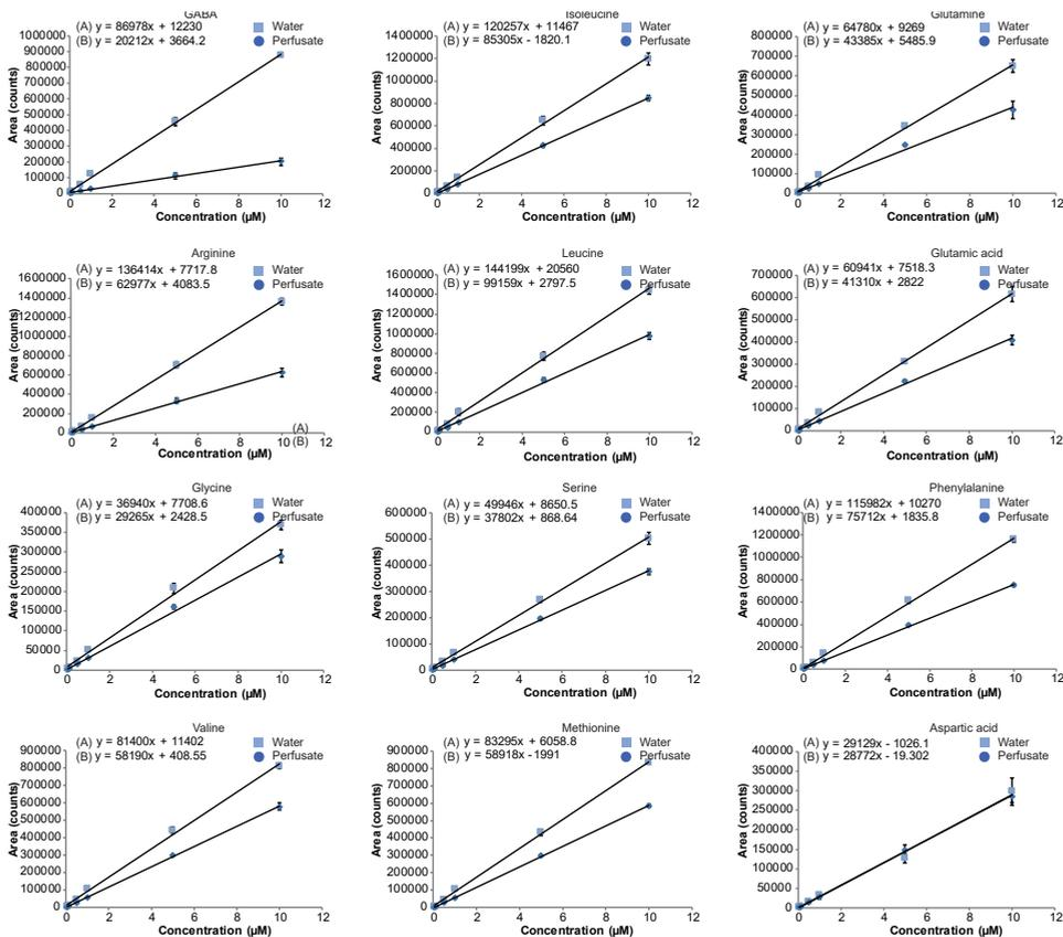
**Figure 3.** Calibration curves for (A) amino acid standards in water and (B) amino acids spiked in perfusate. The standard concerned is indicated above the Figure. Separation conditions: BGE, 10% acetic acid; sample injection volume 291 nL; ammonium hydroxide (concentration: 5%) pre-injection volume, 12 nL.
