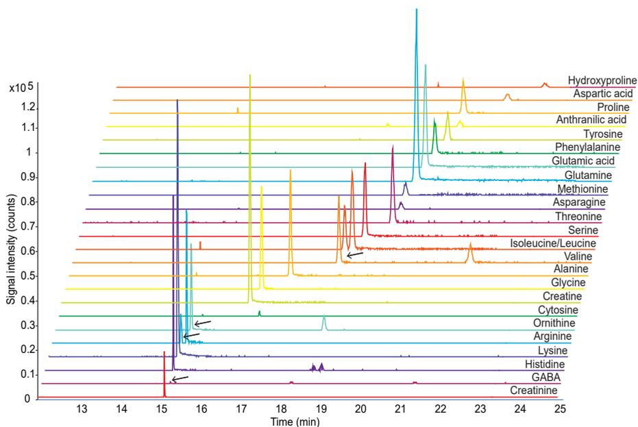
**Figure 4.** Extracted-ion electropherograms obtained by CE-MS from the analysis of endogenous metabolites in basal rat brain microdialysate. Separation conditions: BGE, 10% acetic acid; sample injection volume 291 nL; ammonium hydroxide (concentration: 5%) pre-injection volume, 12 nL.
