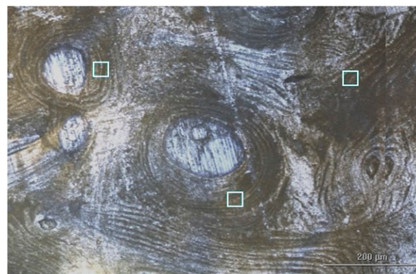
Figure 1. Representative optical micrograph of the cortical bone specimen marked with sites of spectral acquisition.
