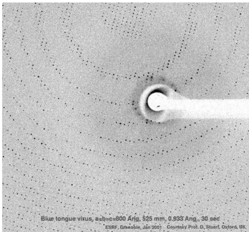
Fig. 5. A zoomed view of a diffraction pattern collected by a MARResearch direct conversion area detector of a Blue Tongue virus crystal (cubic space group,  $800 \times 800 \times 800 \text{ \AA}^3$  unit cell), in a geometry comparable to Fig. 1 (left). Despite the close spacing of the diffraction spots, a very good separation is achieved through the combination of the large size (which also reduces background) and the low point spread of the detector.
