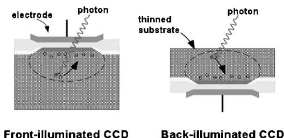
Fig. 4. Front-illuminated CCDs have a lower quantum efficiency than back-illuminated CCDs as in the former a portion of the photons are absorbed by the detection electronics.
