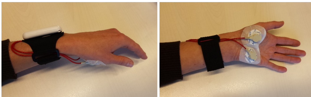
Figure 1. Electrodermal activity (EDA) sensor used in the experiment (EdaMove 4).
