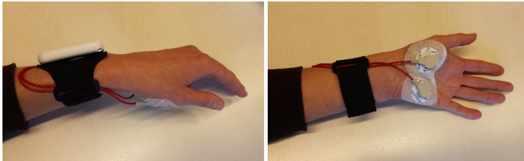
Figure 1. Electrodermal activity (EDA) sensor used in the experiment (EdaMove 4).
