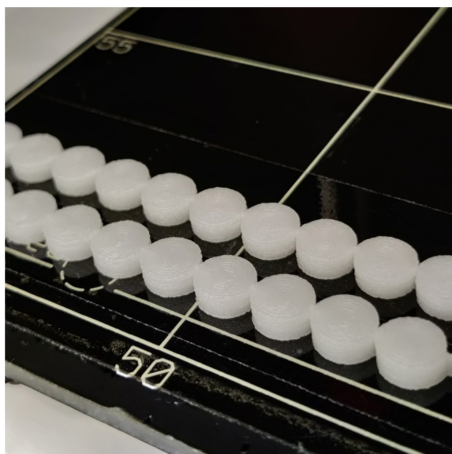
Figure 3 The 3D-printed tablets containing 10 mg sildenafil.
